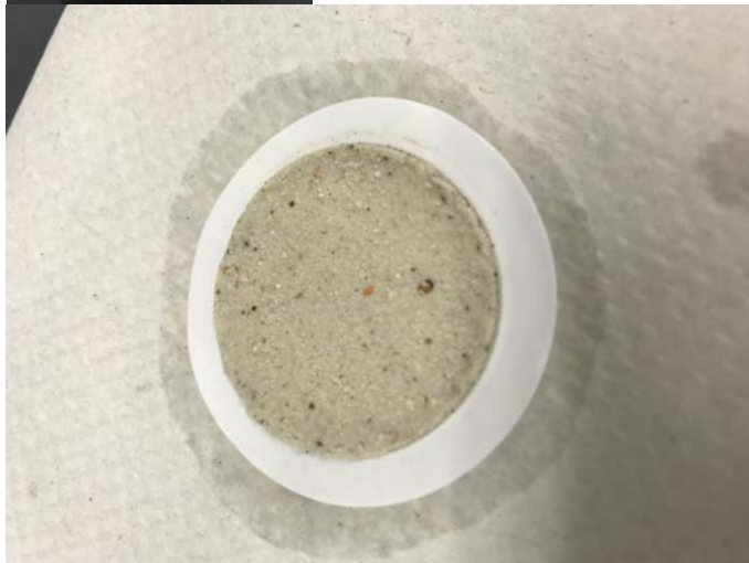
Figures 4 and 5: On the left is a raw influent sample taken on 9-9-2021 at 0452 hours. Note the unusual fine white calcium dirincinoate solids that settled out. On the right is a top view of the solids after they were filtered out from the influent sample.
