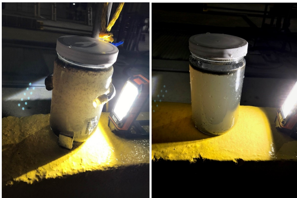
Figures 1 and 2: Samples of JWPCP raw influent taken on 4-14-2021 at 0100 hours. Note the appearance of the samples immediately upon collection (left) and then after 1 minute of settling (right). Note how readily the material floats due to the presence of cationic polymer.
