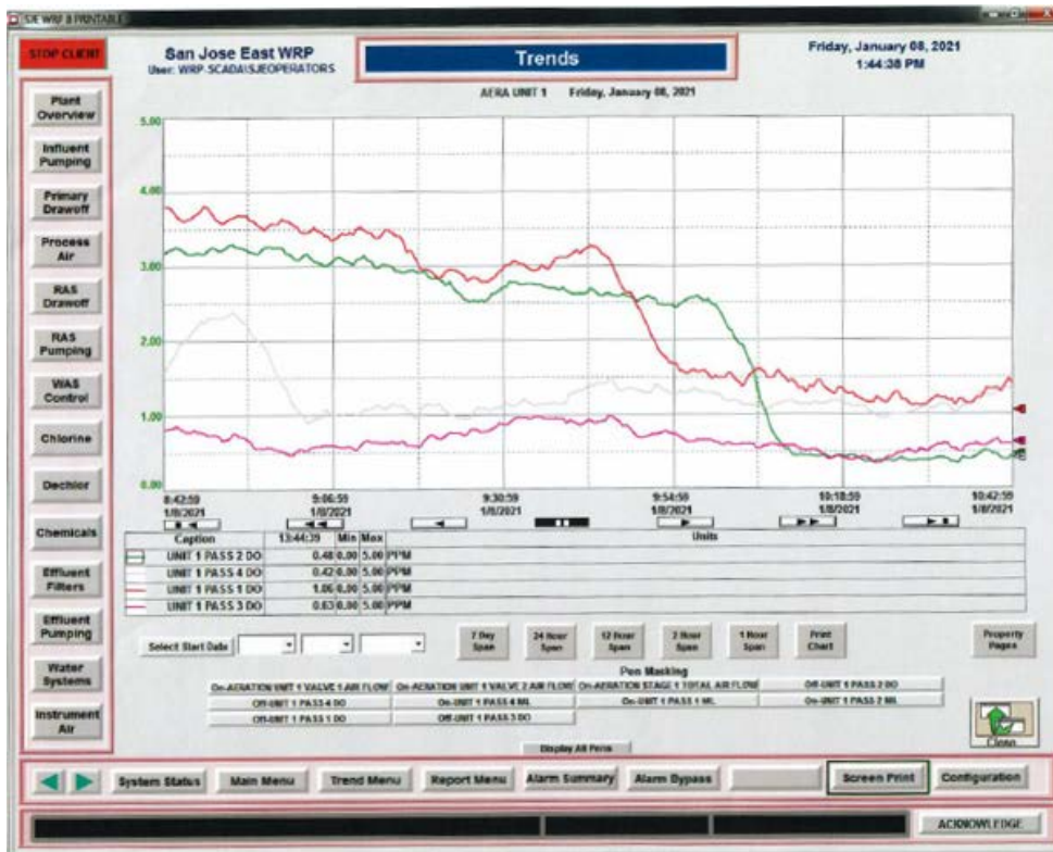
Figure 1: San Jose Creek East WRP dissolved oxygen trend data showing the D.O. drops in the aeration tanks on 1-8-2021 at about 0945 hours.
