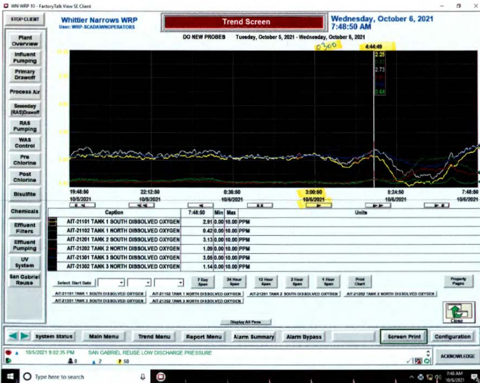
Figure 5: Whittier Narrows WRP aeration tank dissolved oxygen trend data for 10-6-2021. Note the drop off that started at 0445 hours and lasted about 2 hours.
