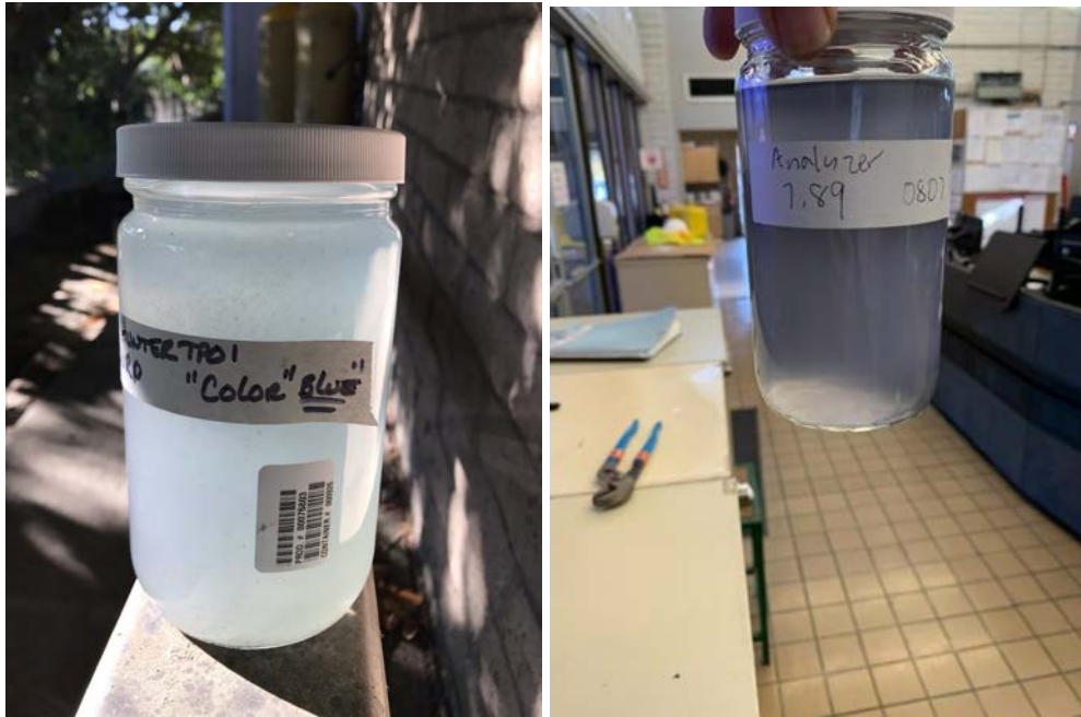
Figures 3 and 4: Los Coyotes WRP raw influent samples taken on 10-10-2021 and 10-21-2021, respectively showing the blue and purple colors reported on those days.
