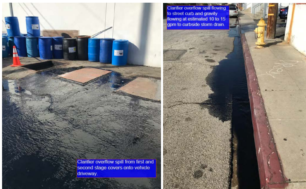
Figures 1 and 2: 11-3-2021, 1015 hours photos of the ongoing overflowing industrial wastewater clarifier into the street gutter, i.e., storm drain, at the Stantex Inc. facility in Vernon.
