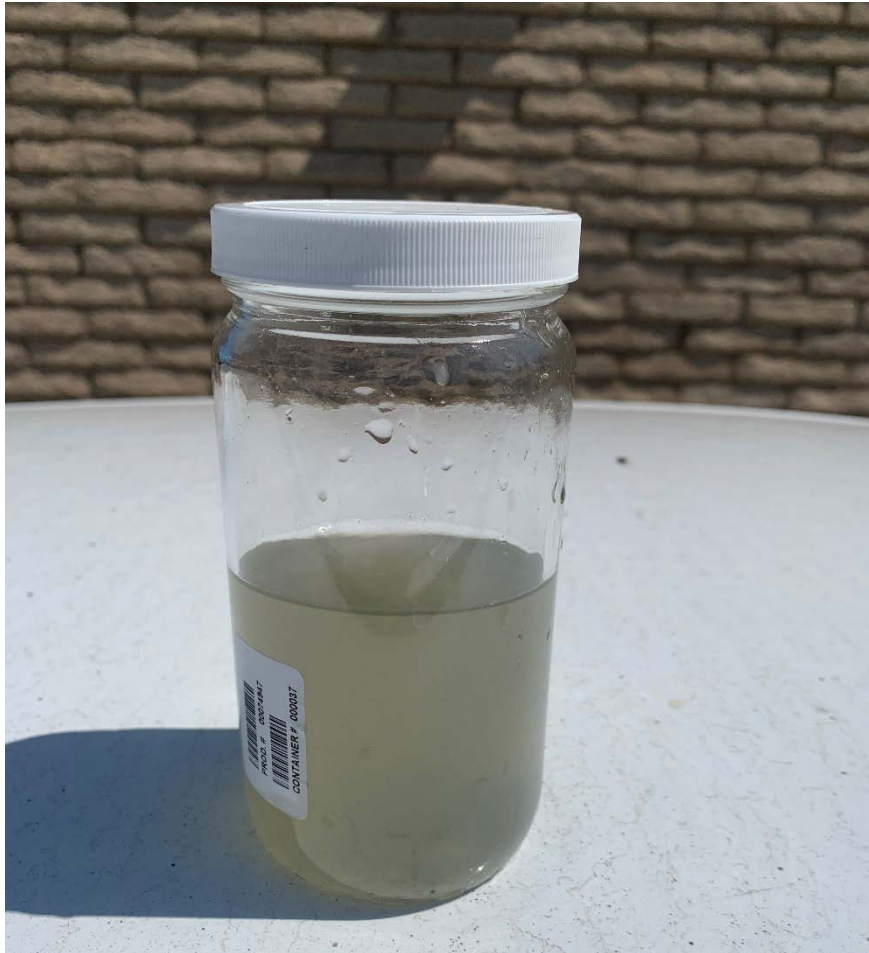
Figure 3: LCWRP raw influent sample taken on 6-26-2021 at about 0915 hours. Note that the sample contains essentially no unusual color.
