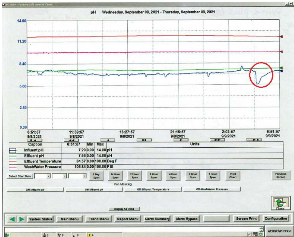
Figure 3: Pomona WRP influent pH trend (blue line) for 0700 hours on 9-8-2021 to 0700 hours on 9-9-2021. Note low pH dip at about 0430 hours on 9-8-2021.
