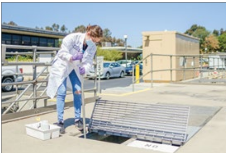
A laboratory technician takes an effluent sample at San Jose Creek WRP
