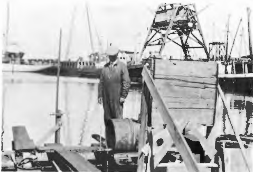
SEWAGE DIFFUSION STUDIES —Floating barge and equipment at Los Angeles Harbor used in determining formulae for predetermining extent of field of contamination over a sewer outlet into seawater. Dr. H. K. Palmer is shown conducting investigation.
