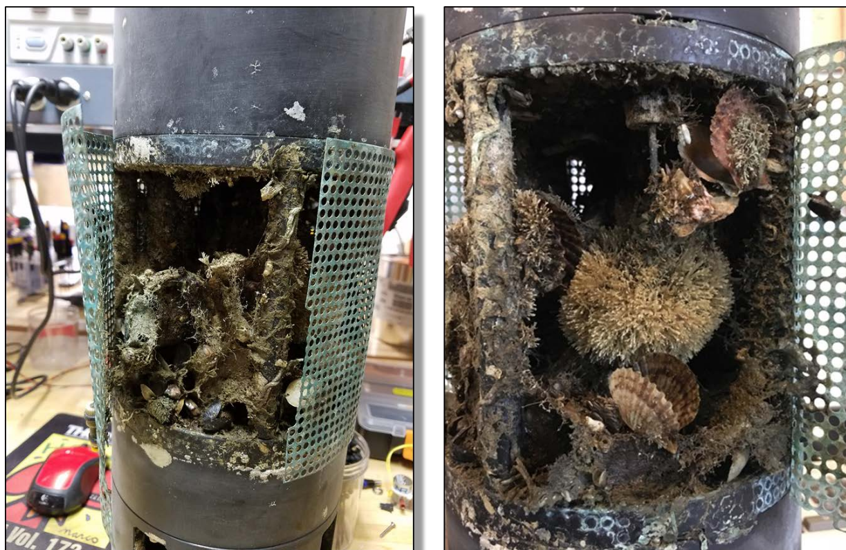
Figure 6 After final recovery from the First Year mooring biofouling on the SAMI pCO 2 sensor was significant
