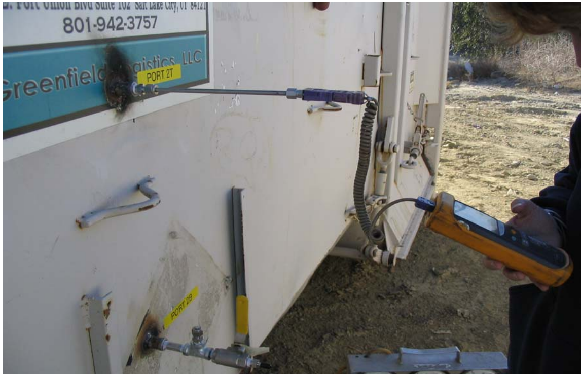
Photo 5 – Interior temperature monitoring
