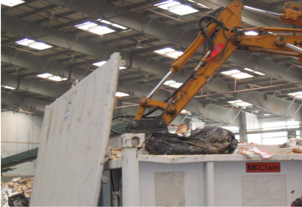
Photo 3 – Refuse is being tamped down in test container with an excavator
