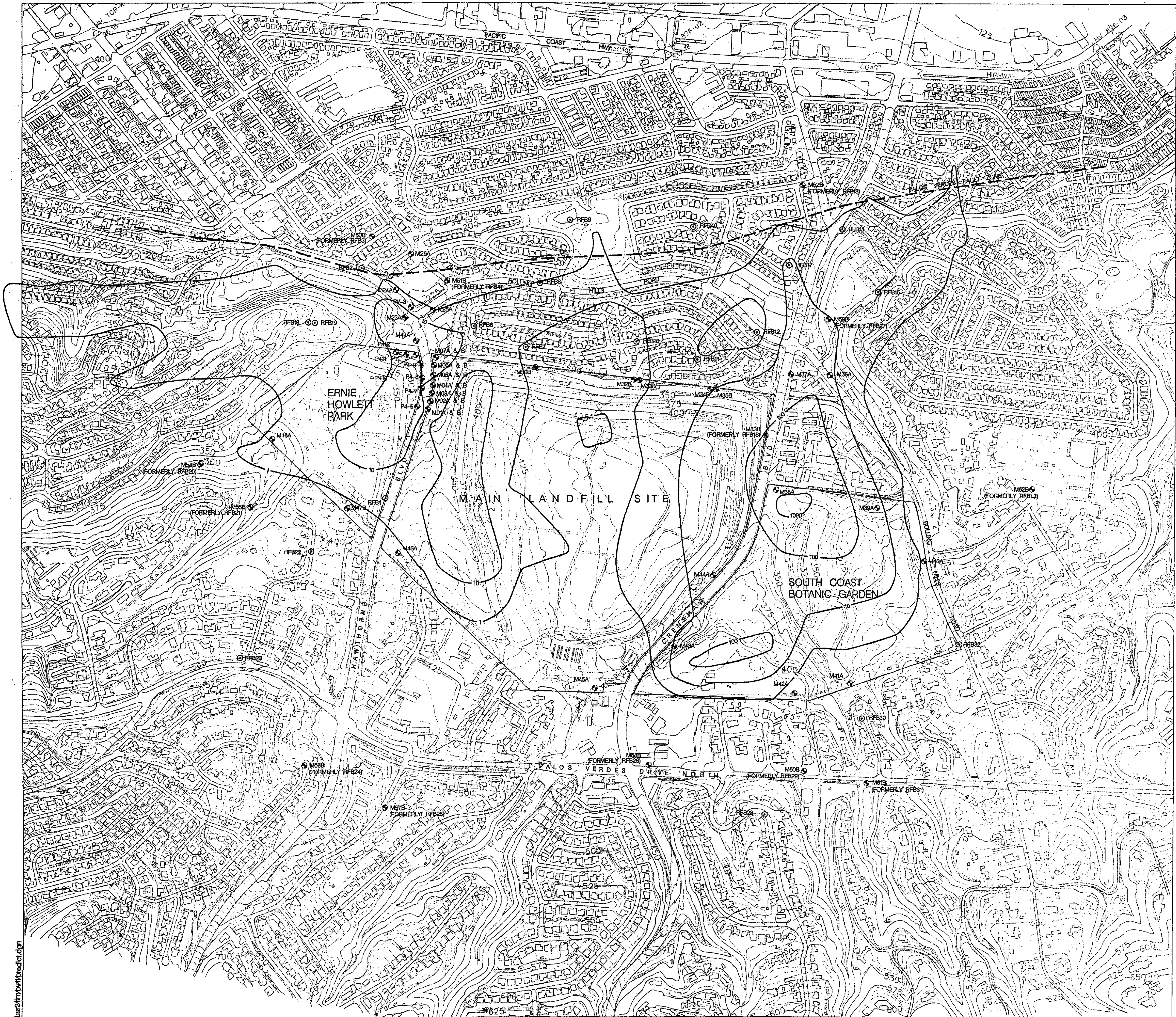
FIGURE G.9e SENSITIVITY ANALYSIS, CASE 9, SIMULATED VINYL CHLORIDE CONCENTRATION AT 200 YEARS
