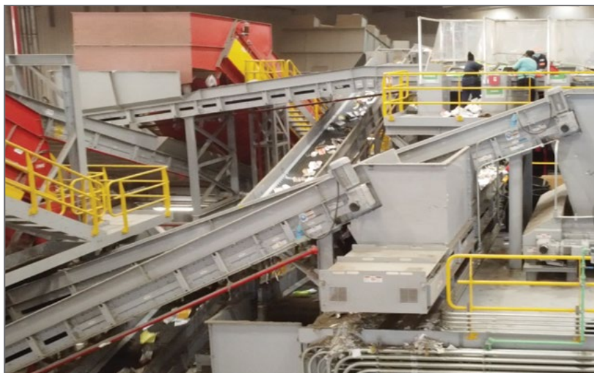
A new automated sorting line has improved cost-effectiveness and increased the purity of recyclables.
