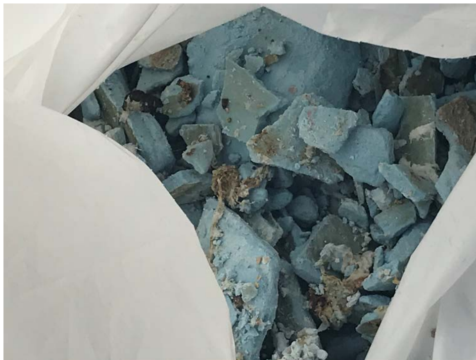
Figure 3: Sample of the blue solids removed from the sewer by City of Lancaster sewer maintenance crews.
