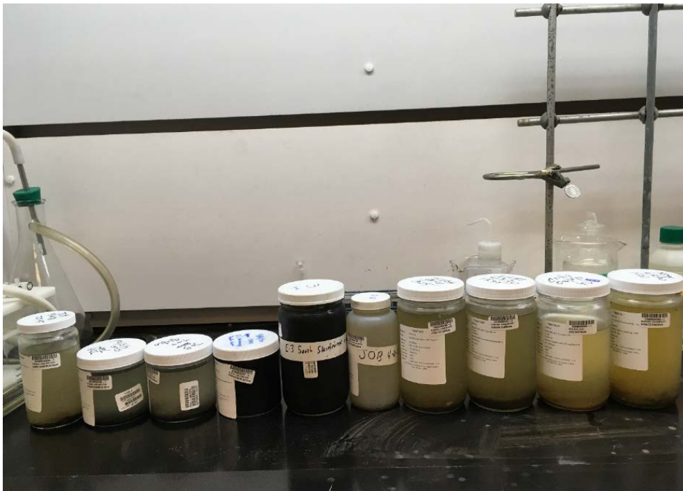
Figure 2: Samples submitted for GCMS and FTIR analysis as part of the JWPCP black solids investigation.
