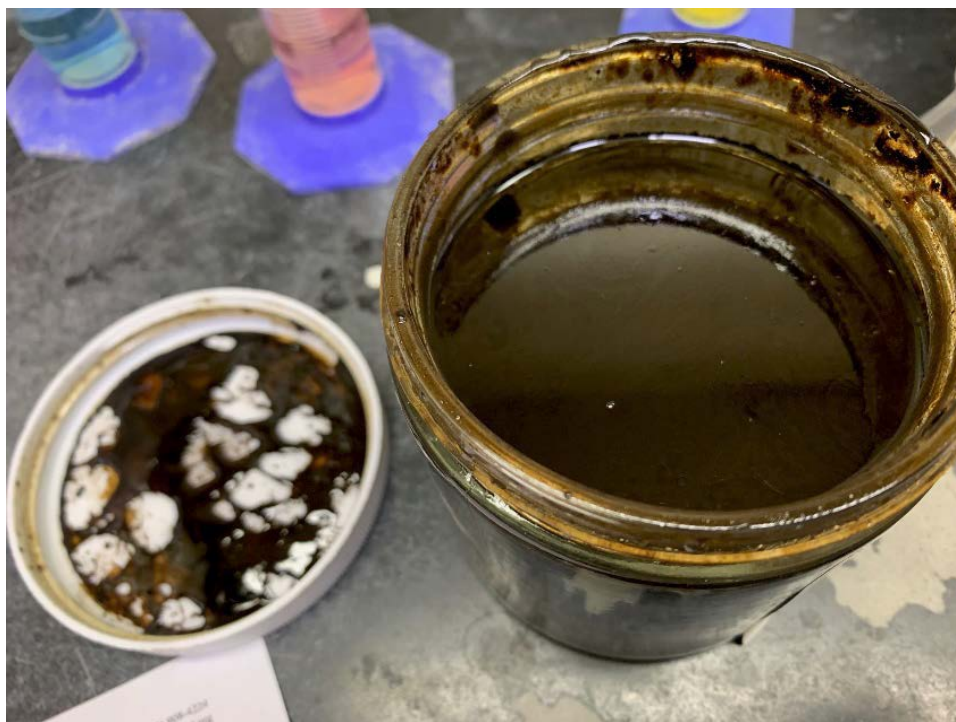
Figure 3: Sample collected from the discrete ISCO sampler at the Phillips 66 oil refinery's legal sample point on 11-24-2020. The sample characteristics were consistent with the oil found at JWPCP and subsequent GCMS analysis confirmed the match.
