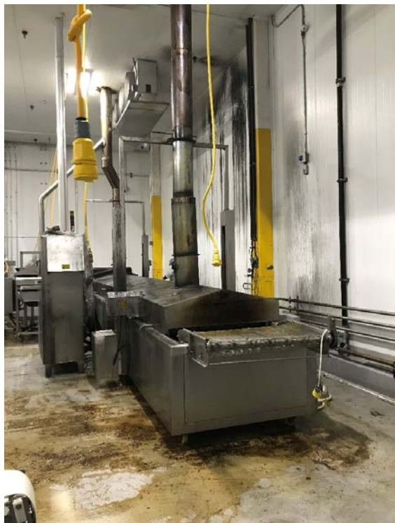
Figures 3 and 4: 12-17-2020 photos showing the stuffed chicken fryer that caught fire and oil residual floating on the top of the wastewater in the industrial wastewater sampling box at Signature Fresh. Note also the oil on the floor next to the fryer.
