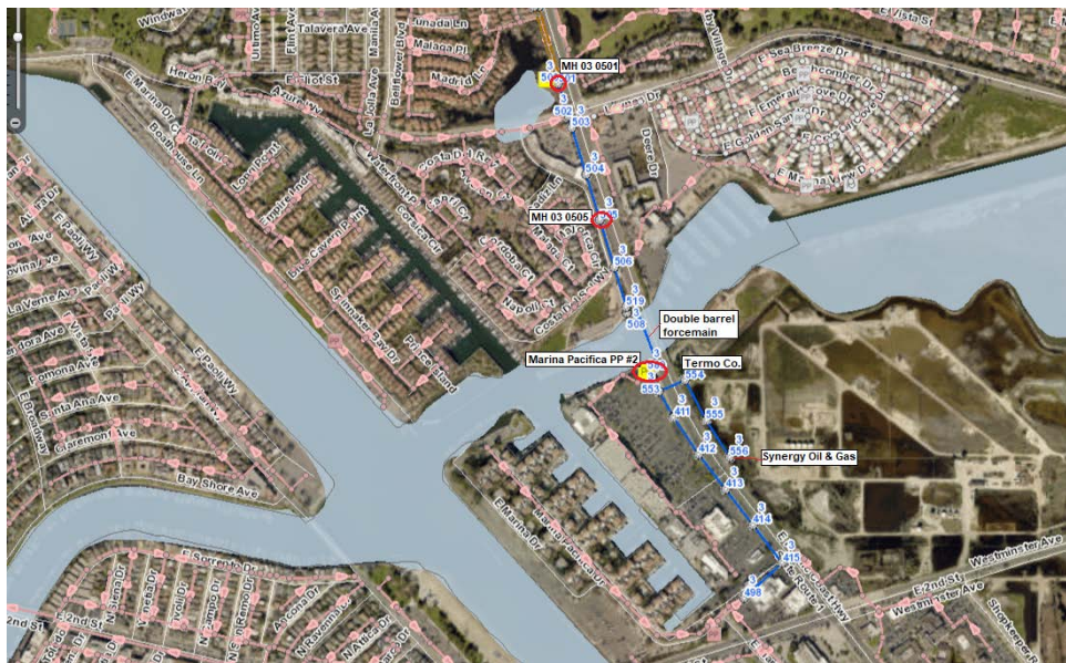
Figure 2: GIS map showing the manhole location of the elevated explosivity on 2-6-2020, MH 03 0505, along with the locations of the upstream pumping plant, and two large oil field production operations that discharge to the sewers in this area.
