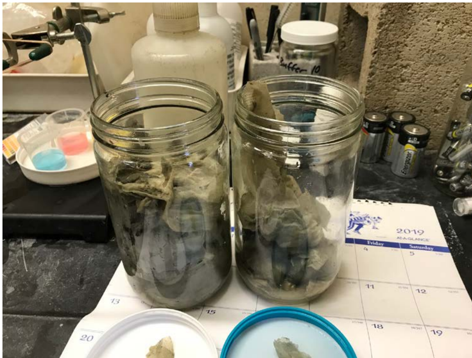
Figure 1: Photos of the “rags” identified as non-woven wipes removed from the sewer at MH 2 2128 on 3-9-2020.
