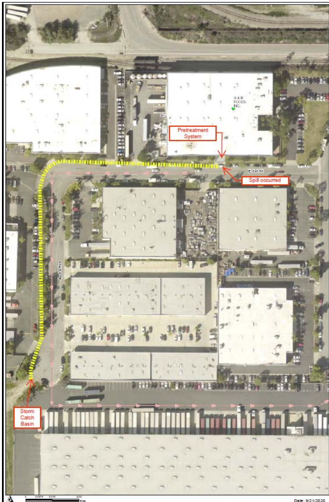
Figure 1: Spill location and the route the spilled wastewater took to the storm drain system.
