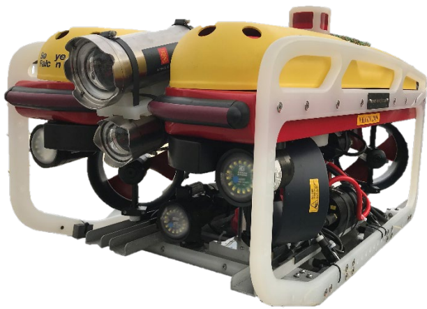
Figure 20: Saab Seaeye Falcon used during the outfall survey.
