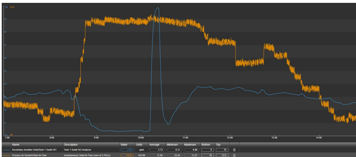
Figure 26. WNWWRP Aeration Unit 1 DO and Total Air Flow November 2, 2023
