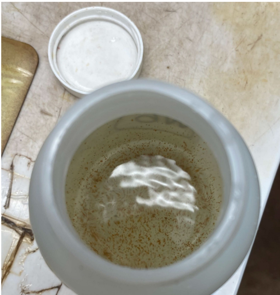
Figure 2: Retain Sample showing solids containing copper at 47mg/l from discharge batch 676
