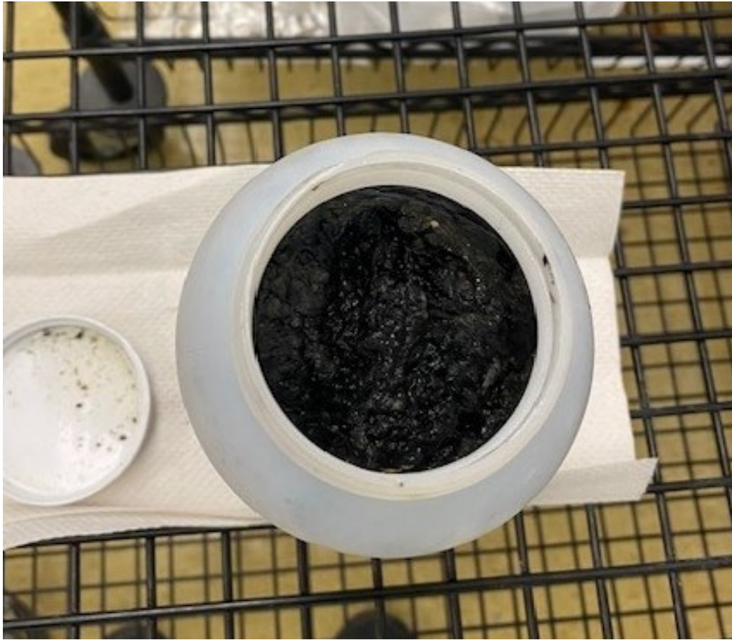
Figure 5. Gelatinous solids from the J.O.'A' Inlet to the headworks
