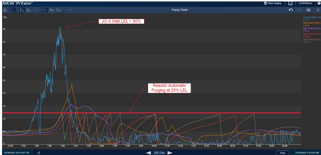
Figure 4. PI Vision chart displaying J.O. “A” Inlet and Reactor combustibility gas levels on August 19, 2023.
