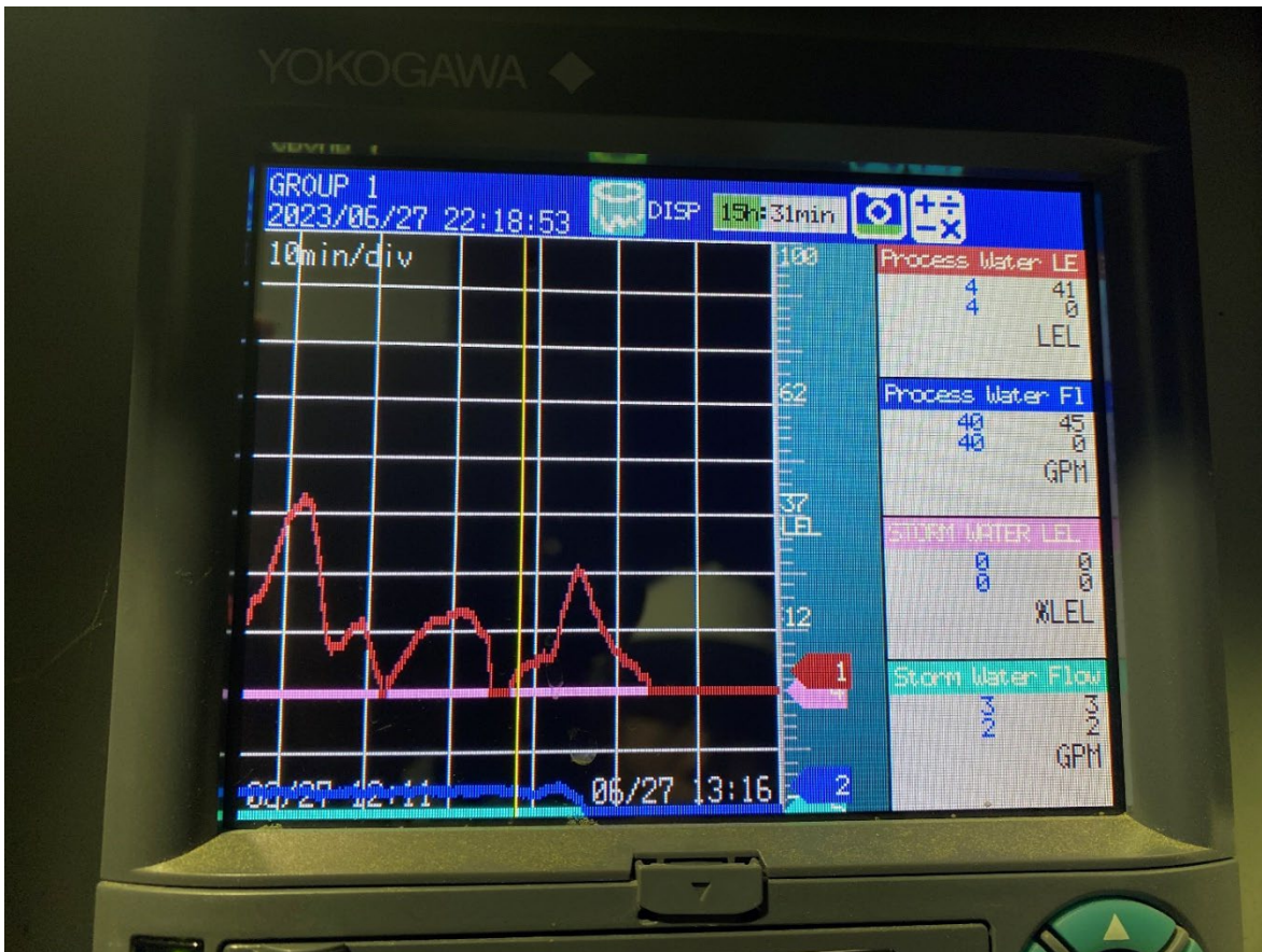
Figure 18. Equilon Enterprise LLC dba Shell Oil Products monitoring equipment. Trend indicates LEL exceedance prior to wastewater impoundment and notification. Trend timespan is June 27, 2023, 133-1243 hour.
