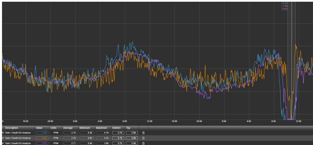
Figure 25. OSI PI Graph WNWRP D.O. at Aeration Units Oct. 30, 2023
