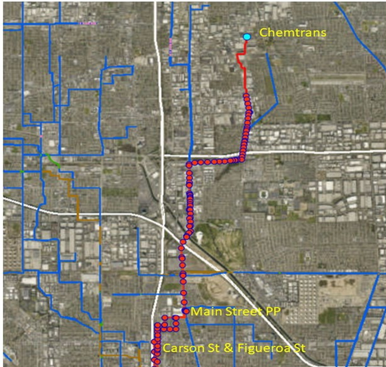
Figure 3. GIS map of the local and Districts' sewer downstream of Chemtrans
