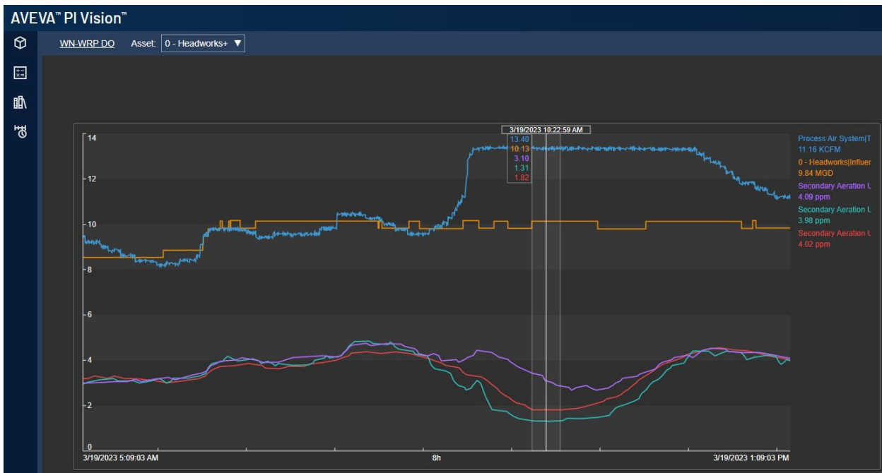
Figure 1. WNWRP Process Air, Headworks Flow & Aeration Units D.O.
