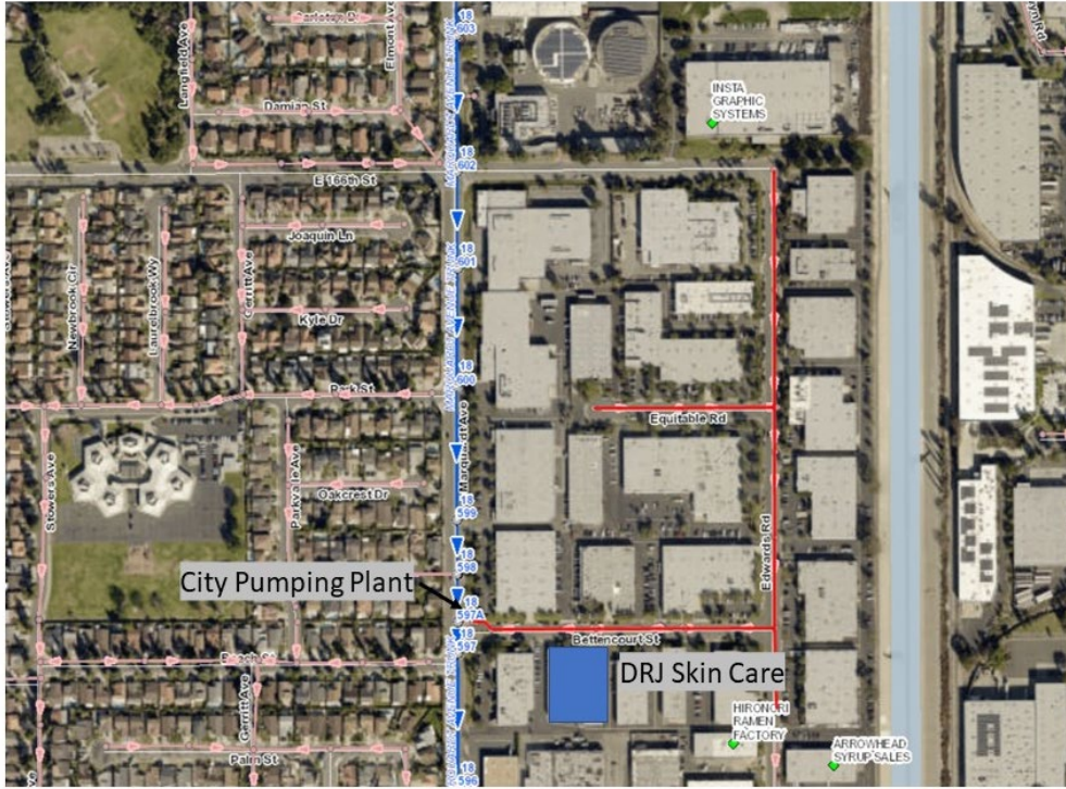
Figure 6. GIS map showing the City of Cerritos Pumping Plant and the upstream sewer.
