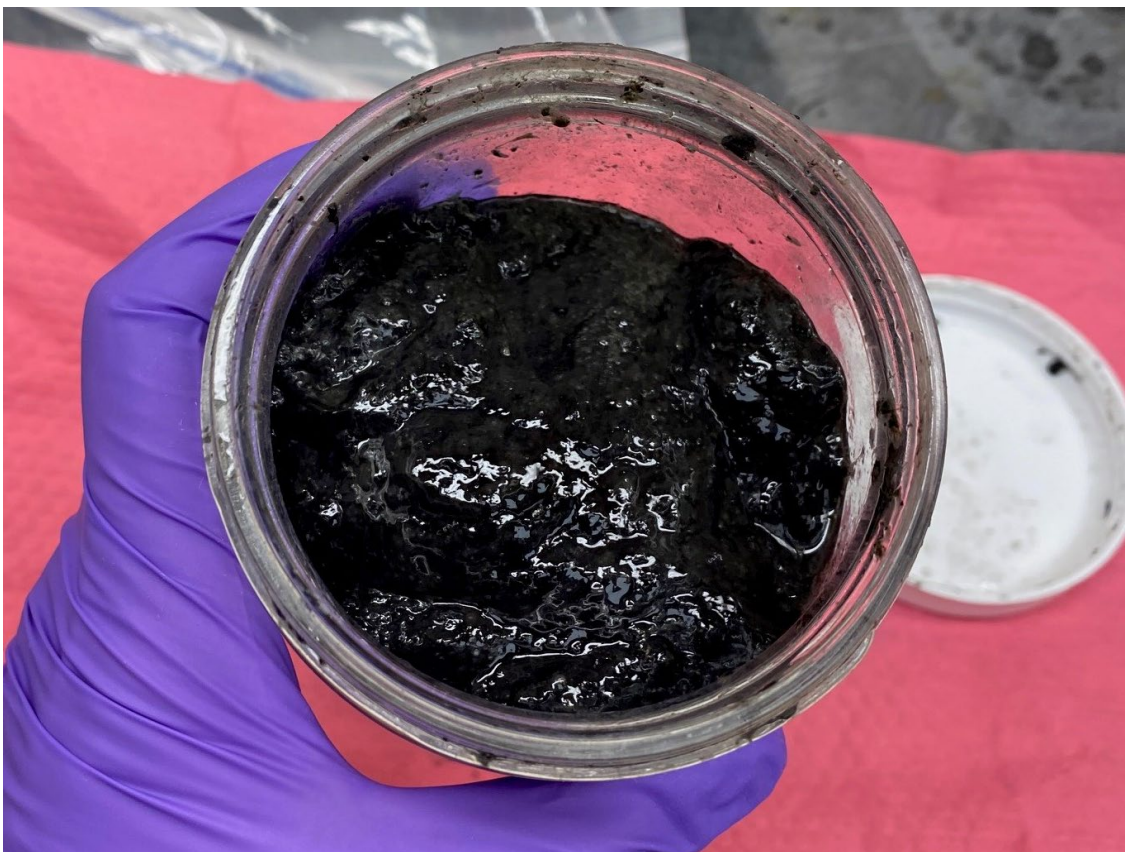
Figure 3: Gelatinous Solids from inlet works
