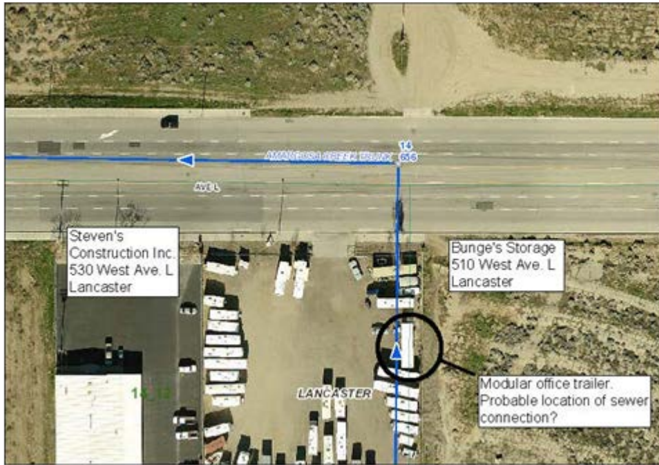
Figure 6: Satellite photo from Sanitation Districts' GIS showing where a modular office trailer was found illegally connected to the adjacent Amargosa Creek trunk sewer line.
