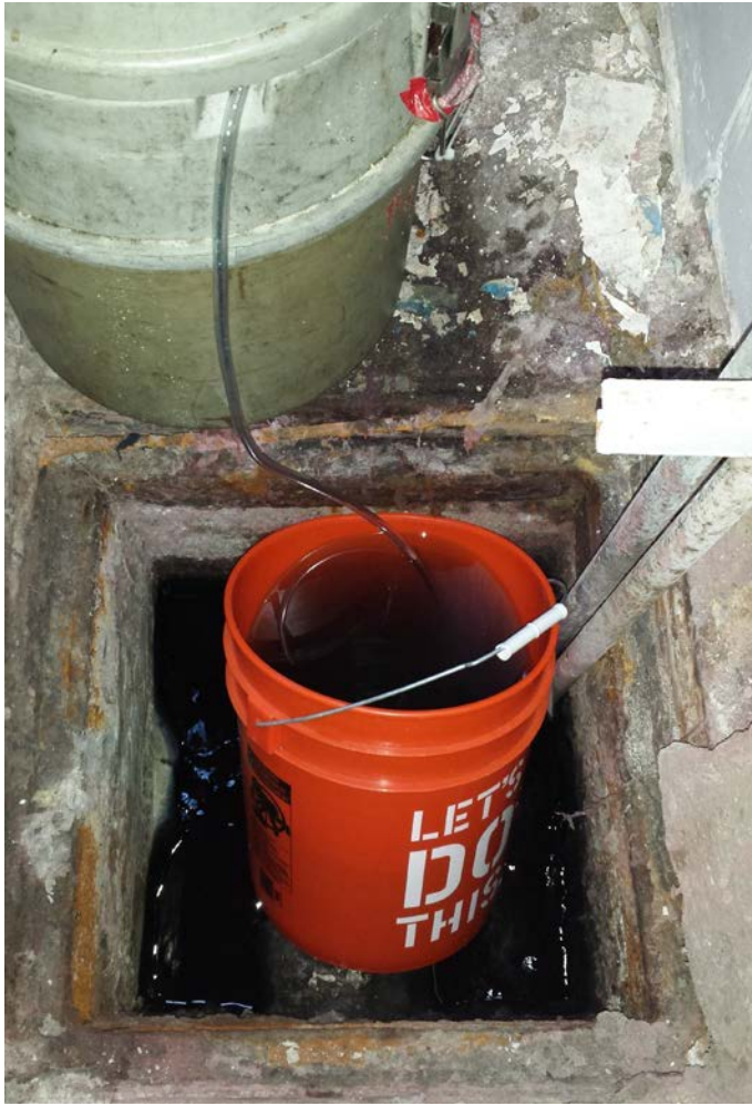
Figure 2: photo of Districts' automatic Isco sampler in position at the sample box of United Dye & Wash on 10-7-14. Note that a bucket of water has been placed inside the sample box such that no sample of the actual water being discharged is being taken.
