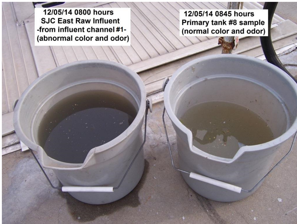
Figure 5: Photo of samples taken at SJC-East WRP on 12-5-14 to compare the unusual dark colored raw influent to normal colored sewage.
