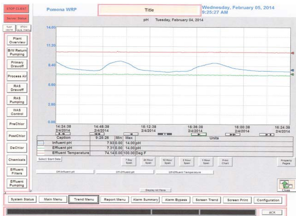
Figure 1: Influent pH screen grab chart from the Pomona WRP on 2-4-14. The blue line indicates the two high pH periods.
