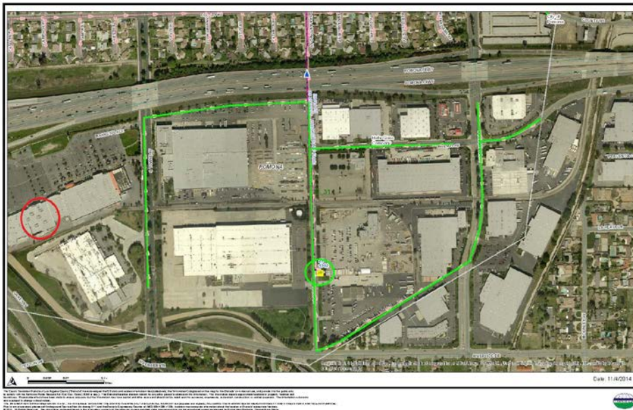
Figure 3: Districts' geographic information system (GIS) photo map showing the relatively limited area influent to the Pomona Pumping Plant No. 4. Note, circled in red, the vacant commercial property at 2727 S. Towne Ave. that was identified as the flow source.
