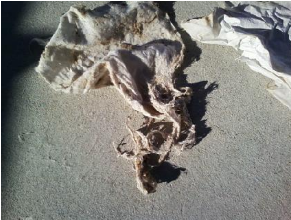
Figure 12: 12-29-14 photo of plastic-based disposable wipe removed from the flex rake screening system at Lancaster WRP. Note how similar the wipe appears to cloth when encountered at this location.
