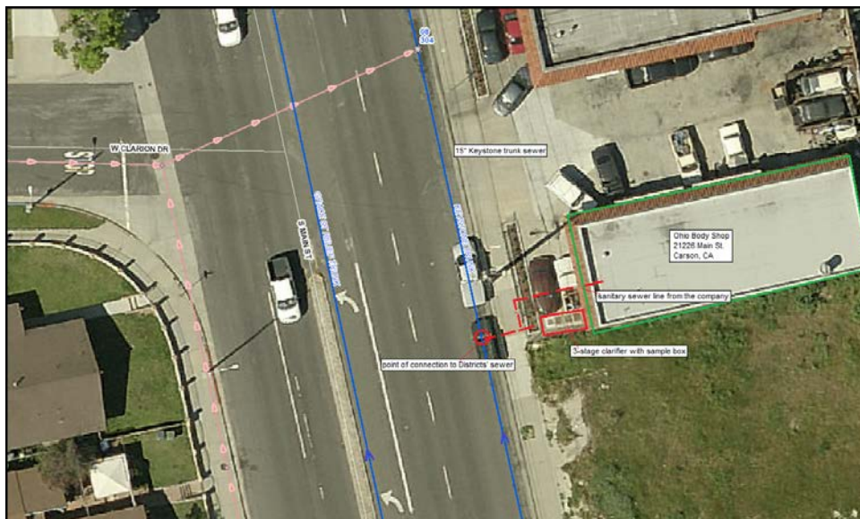
Figure 1: Diagram of the Ohio Body Shop direct connection to the Districts' 15" Keystone trunk sewer in Carson.
