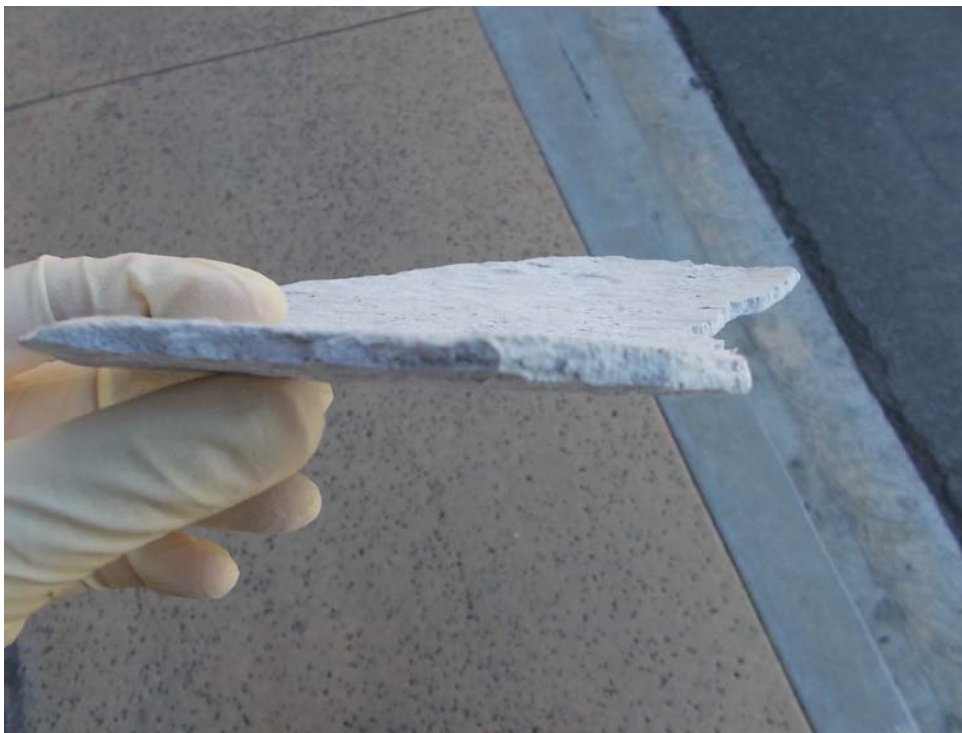
Figure 4: Sample of the scale like material found at MH 29 in the Puente Trunk on 7-21-14.
