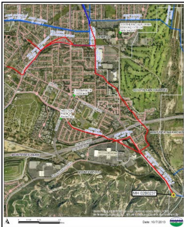
Figure 2: GIS Map indicating the Districts' trunk sewers and Montebello local sewers tributary to the siphon
