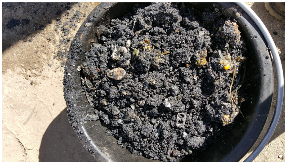
Figure 3: Sand and grit removed from MH B0237 on 11-13-15. Note that these particular cleanings did not have much grease present.
