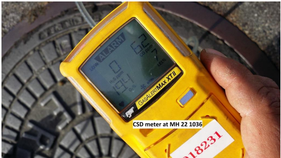
Figure 9: Districts' sewer maintenance crew 4-gas meter indicating 62 ppm of carbon monoxide in the headspace gas in Irwindale trunk sewer Manhole 22 1036.
