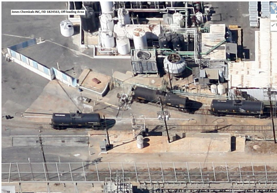
Figure 4: Google Maps Satellite view further zoomed in showing the rail spur ending just below the cooling towers and tank farm where the tanker car overran the end of the track causing the spill.
