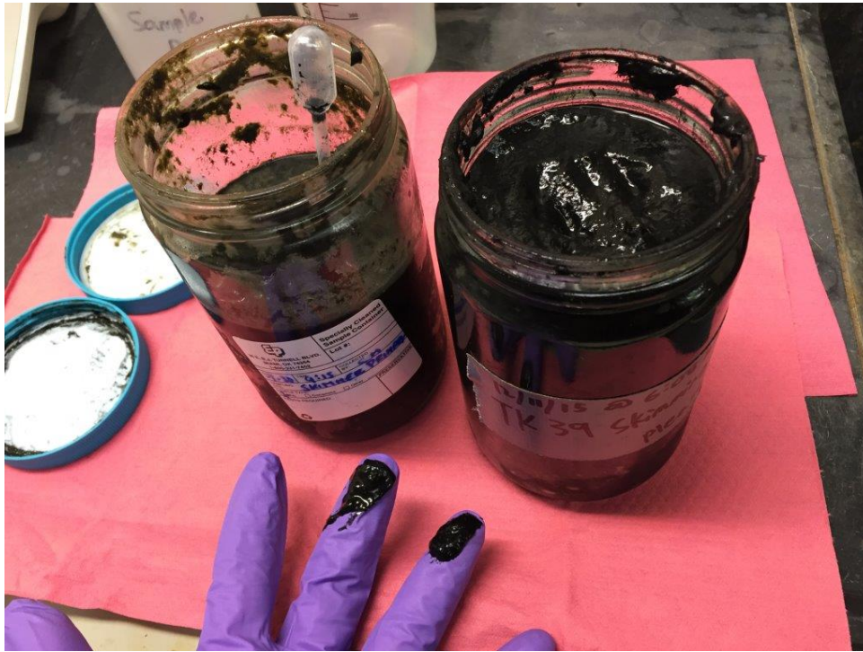
Figure 3: Visual comparison of 7-30-15 and 12-11-15 samples of JWPCP primary skimmings solids both reported as having a black “oily” appearance. Note their similarity.
