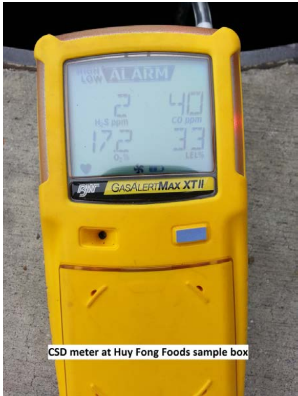
Figure 10: Districts' 4-gas meter indicating 40 ppm of carbon monoxide, along with elevated LEL and hydrogen sulfide concentrations in the headspace gas of the industrial wastewater sampling box at Huy Fong Irwindale, LLC in Irwindale.
