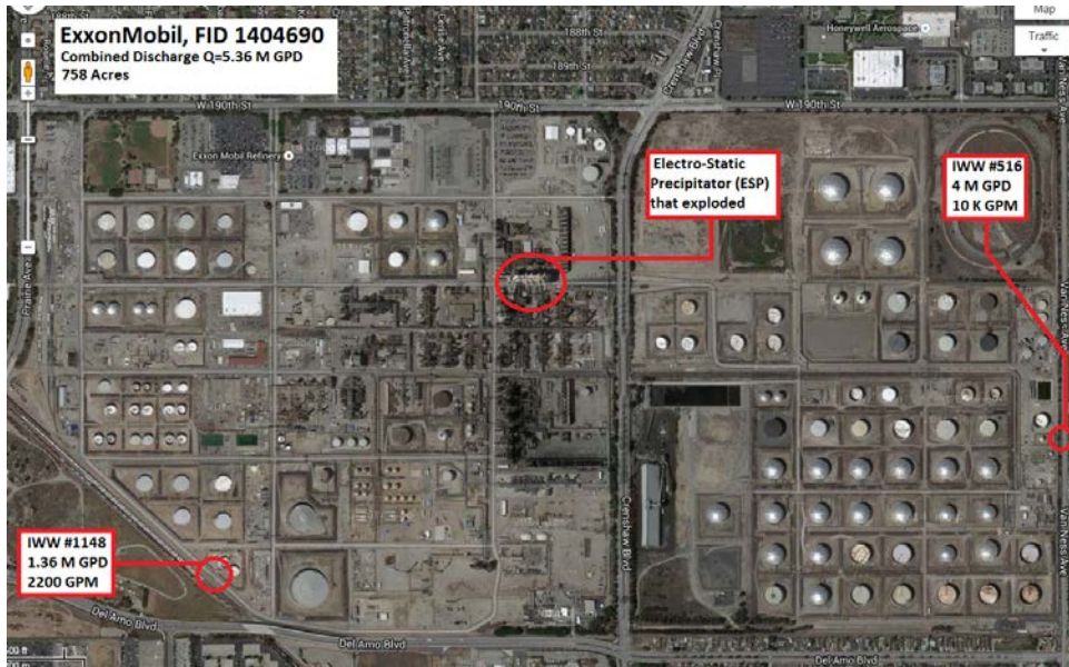
Figure 3: Google maps aerial diagram of the ExxonMobil refinery in Torrance. Note the location of the Electrostatic Precipitator (ESP) unit where the explosion occurred in relationship to the two permitted industrial wastewater outfalls at the facility.
