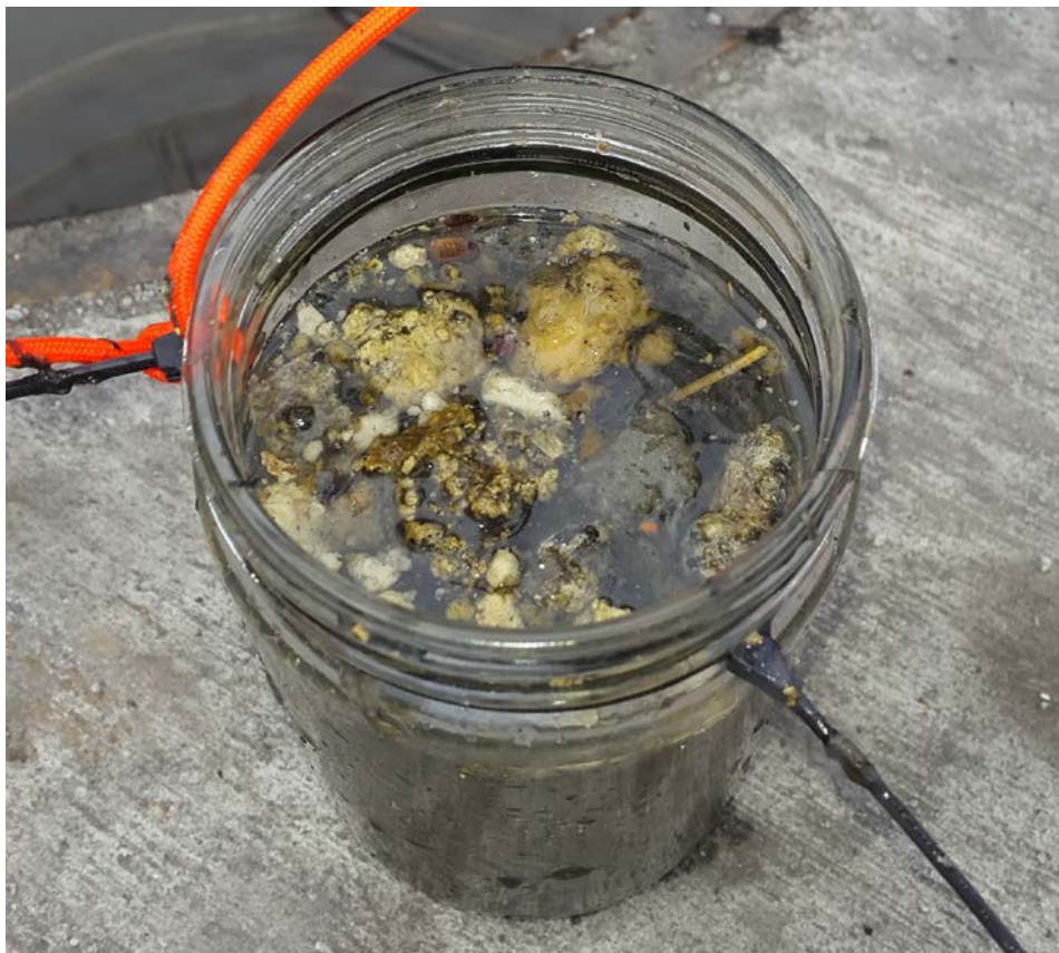
Figure 7: Sample of the FOG removed from MH 08A0470 on 6-12-15.
