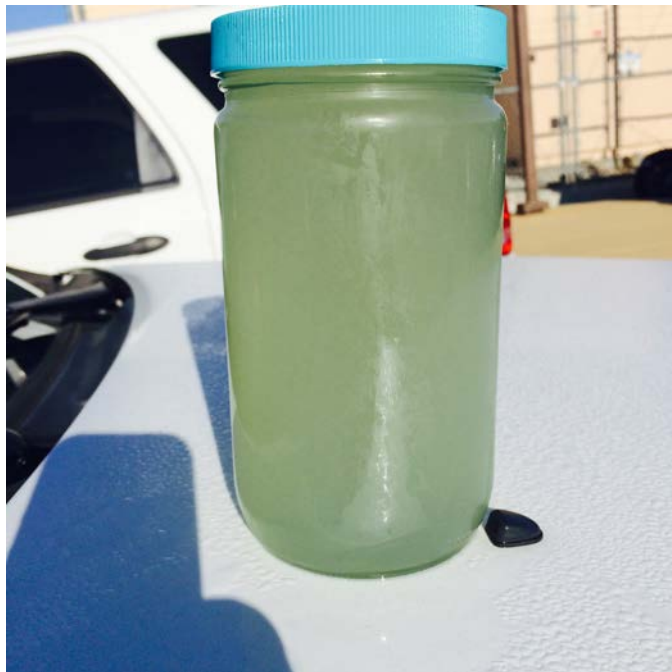
Figure 10: Green color sample taken on 2-27-15 from a Lancaster WRP primary tank.
