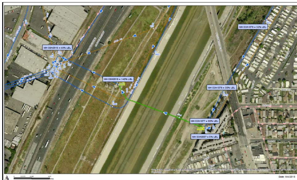
Figure 4: Sewer diagram indicating I.W. inspector explosivity levels found at various manholes during their investigation on 9-2-15.
