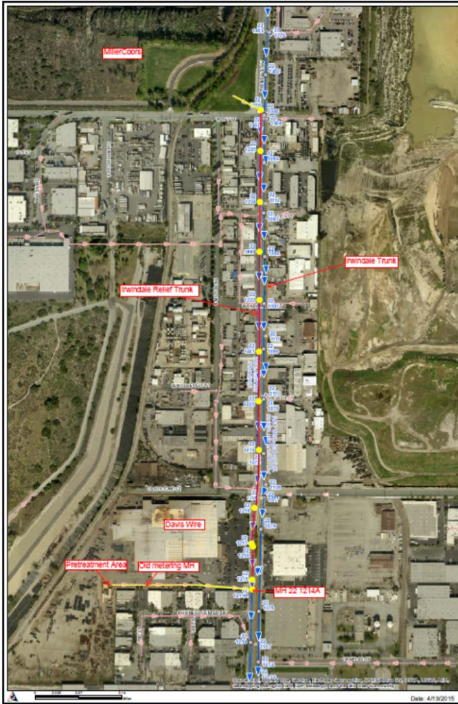
Figure 6: GIS diagram showing the location of manhole 22 1214A where calcium sulfate scale was found.
