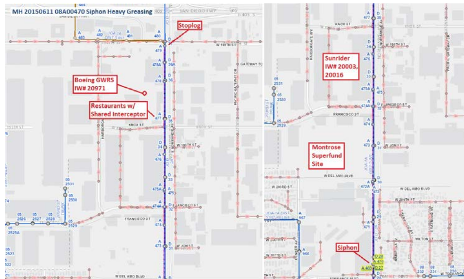
Figure 5: Sewer line diagrams indicating the area upstream of MH 08A0470 where heavy greasing was found on 6-11-15 by a Districts' CCTV crew.
