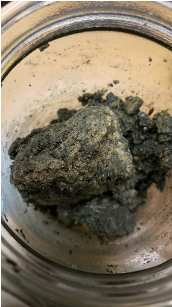
Figure 6: Fist sized chunk of grease removed from MH H 242A on 8-17-16.
