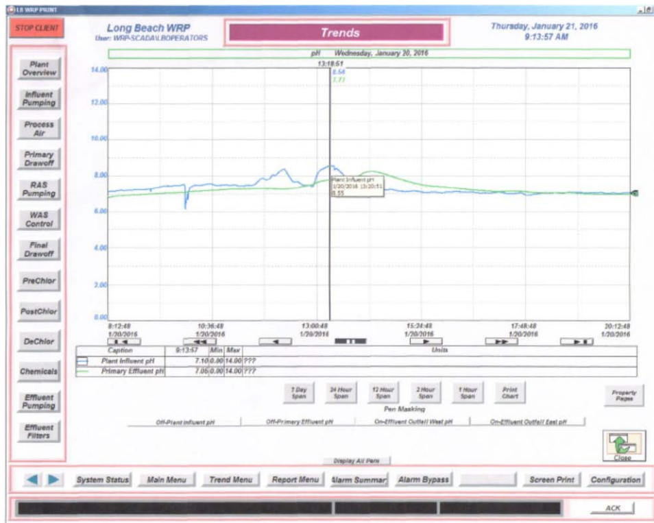
Figure 11: LBWRP influent pH trend chart on 1-20-16 from 0812 hours to 2012 hours.
