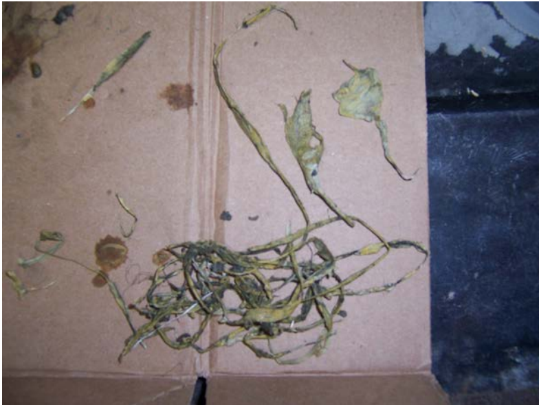
Figure 3: Photo of the materials reported to be elastic or rubber bands. Note the materials are in fact not elastic and can be “unrolled” to reveal their true identity as the remnants of flushable wipes.
