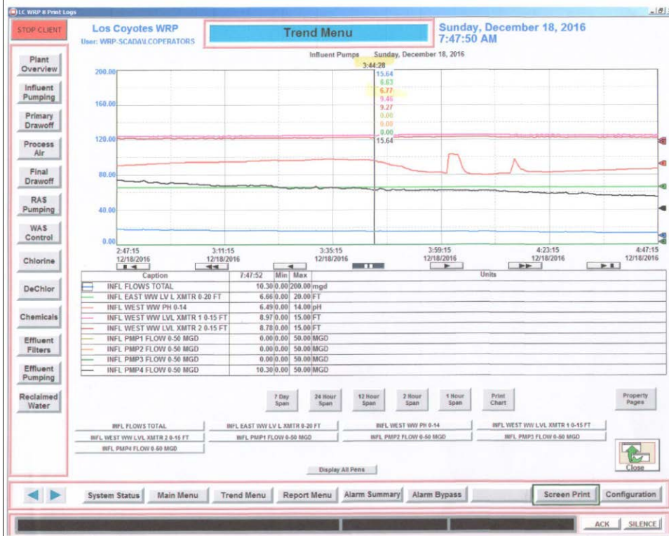
Figure 4: LCWRP screen shot indicating the influent trend pH (red line) during the early morning hours of Sunday, 12-18-16. The data indicates the normal pH trend was first disrupted at 0345 hours. The normal pH trend was regained by 0500 hours.
