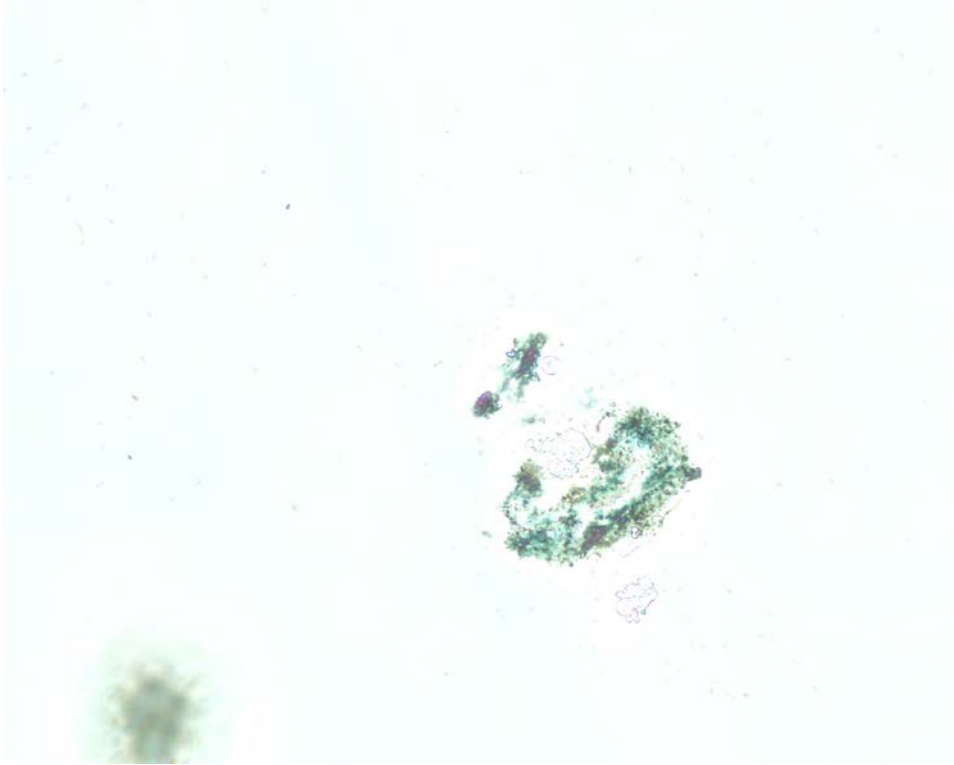
Figure 3: 20X microscope image of blue-green material in secondary effluent.
