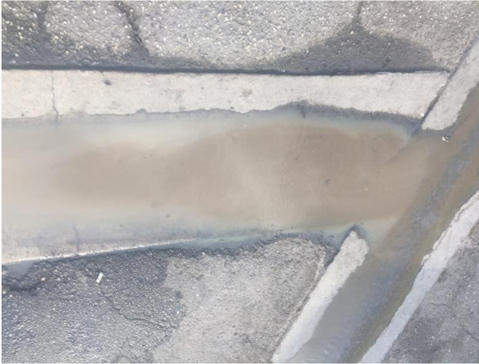
Figure 2: Photo of the contaminated water in a driveway swale sent to Boyd by the anonymous complainant. Note the color matches that expected of water contaminated with emulsified grease.
