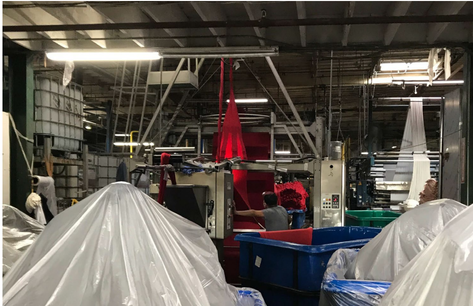
Figure 3: Picture taken at Tri-Star Dyeing & Finishing on February 22, 2022 showing an example of the red fabric being processed that likely caused the February 21, 2022 red color incident at the Los Coyotes WRP.
