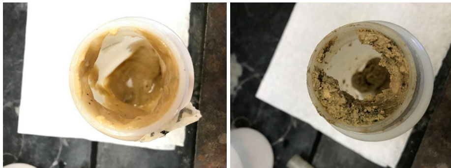
Figures 3 and 4: Grease Samples taken from the local line sewer just downstream of Evans Foods and from MH 15 0057. Note the similarity, though the sample from MH 15 0057 is more weathered and contains mixed in grit from the sewers.
