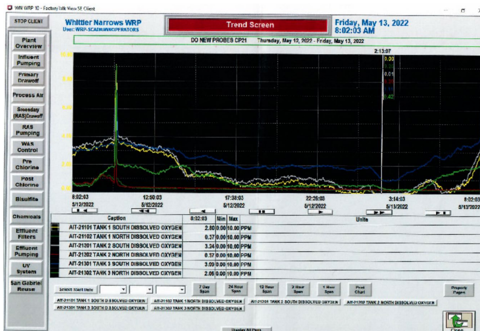
Figure 2: WNWRP control system screen shot showing dissolved oxygen levels in the secondary aeration tanks on May 12-13, 2022.
