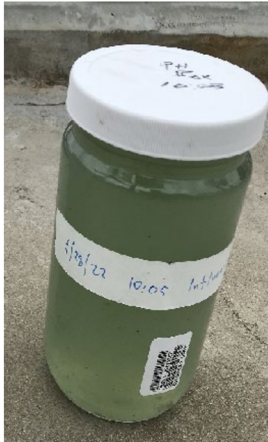
Figure 8: LCWRP raw influent sample taken on 4-28-22 at 1005 hours. Note the blue-green color.
