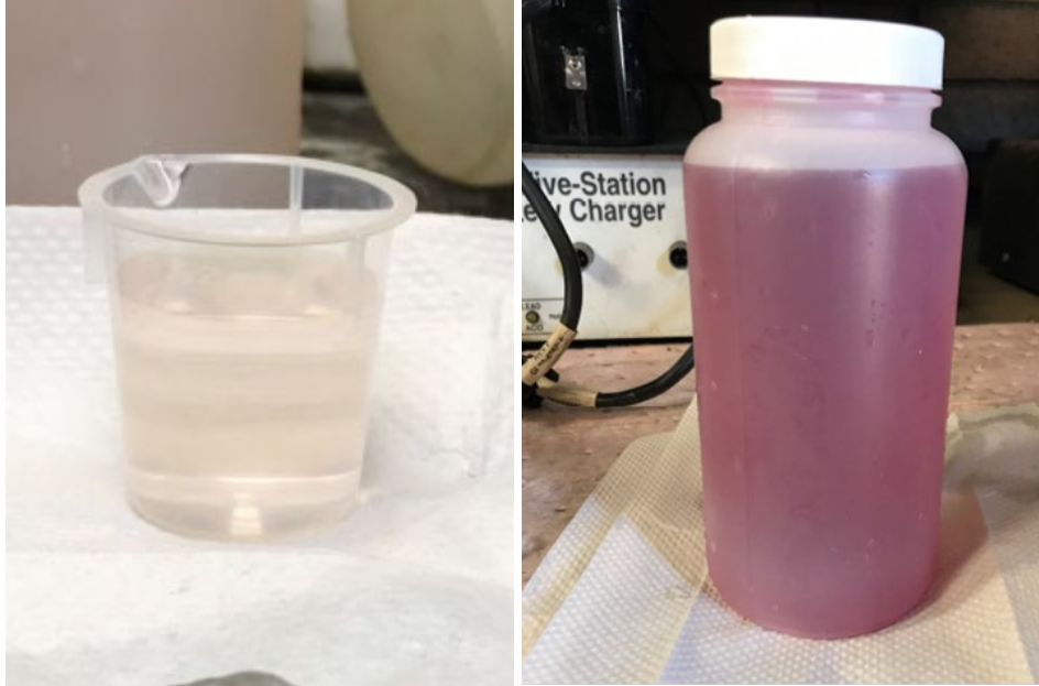
Figures 1 and 2: Sample on the left is that taken from the primary channel at SJC West WRP at 1000 hours on September 14, 2022, and that on the right is a sample of wastewater taken from the batch treatment tank at Danco Anodizing on September 14, 2022, at 1030 hours. Note the light red tint in the WRP sample and the similar, but much darker color in the Danco sample.
