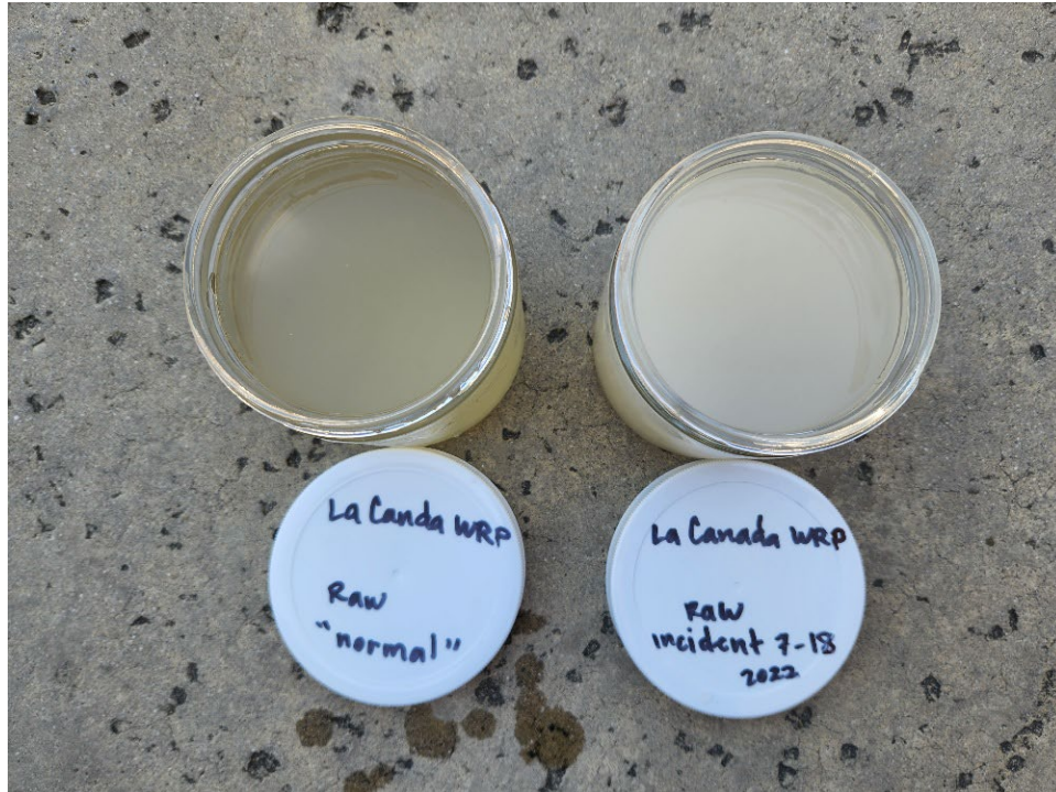
Figure 4: Photo showing a color comparison of “normal” plant influent at the La Cañada WRP vs. that seen when the white color was entering the WRP on 7-18-22.
