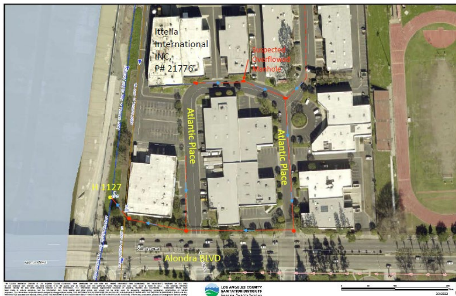
Figure 1: Geographic Information System based annotated diagram of the private sewer line system (red lines) in the City of Paramount where an SSO occurred on 3-1-22.
