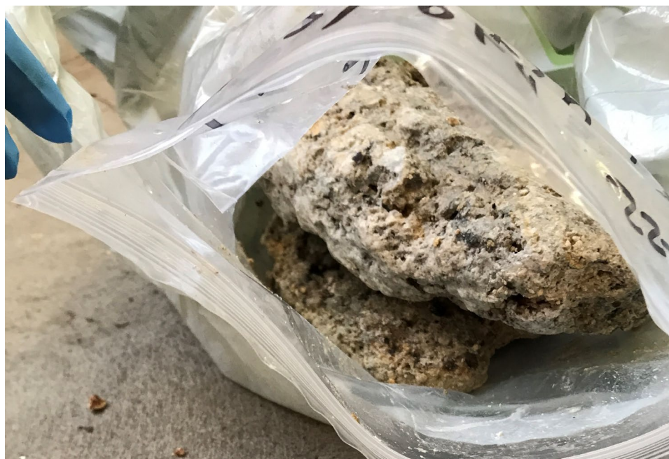
Figure 1: Sample of grease from the siphon structure at manholes 18 0434A and 18 0434.
