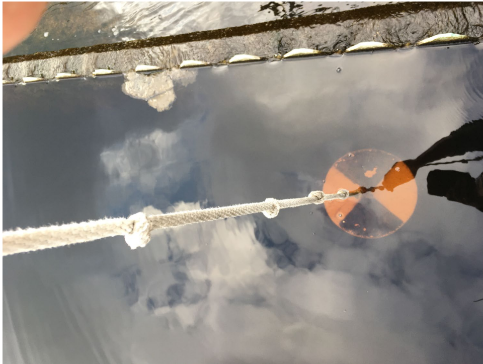
Figure 2: Los Coyotes WRP Forebay on 2-21-22. Note the red color as shown against the white Secchi disc surface.
