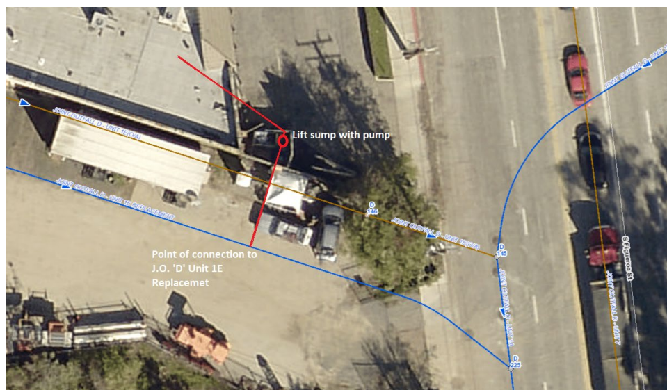
Figure 4: Diagram showing the private lateral sewer line that flows from the strip mall/plaza to J.O. 'D' Unit 1E via a private sewer lift station.
