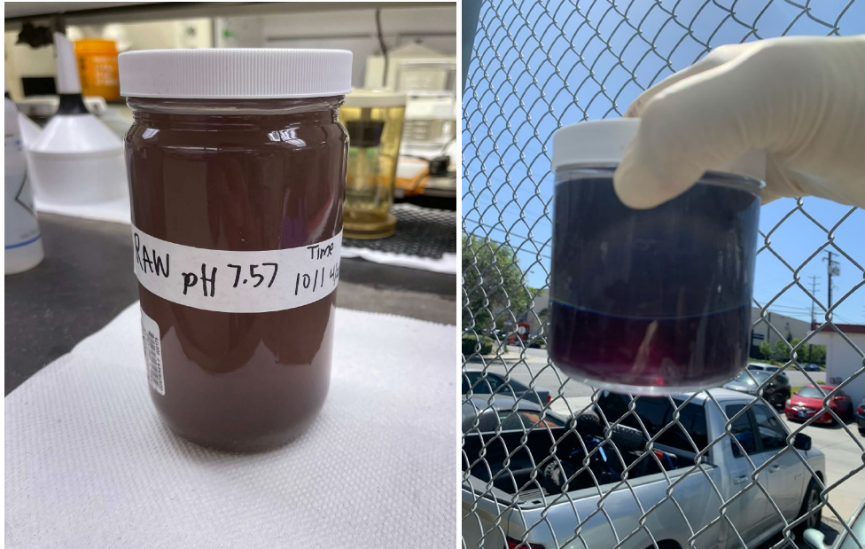
Figures 5 and 6: On the left is the LCWRP influent sample taken on 4-21-22 at 1011 hours. Note the deep purple-brown color. On the right is a sample of the wastewater being discharged that same morning by Tri-Star Dyeing and Finishing. Note the same color as was present at the WRP.
