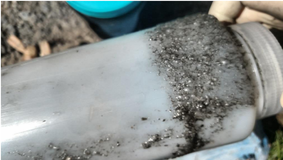
Figure 8: Close up of the foam when skimmed onto a plastic Nalgene bottle. Note how darkly colored the material appears versus when it's seen floating in the tank.
