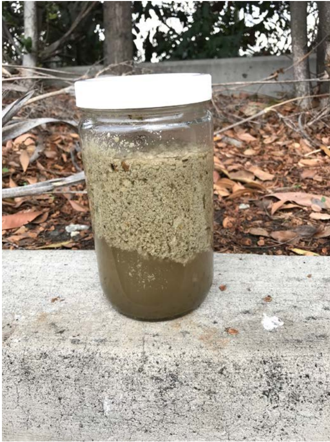
Figure 6: Floating grease in a sample taken from the Coyote Creek pumping plant.
