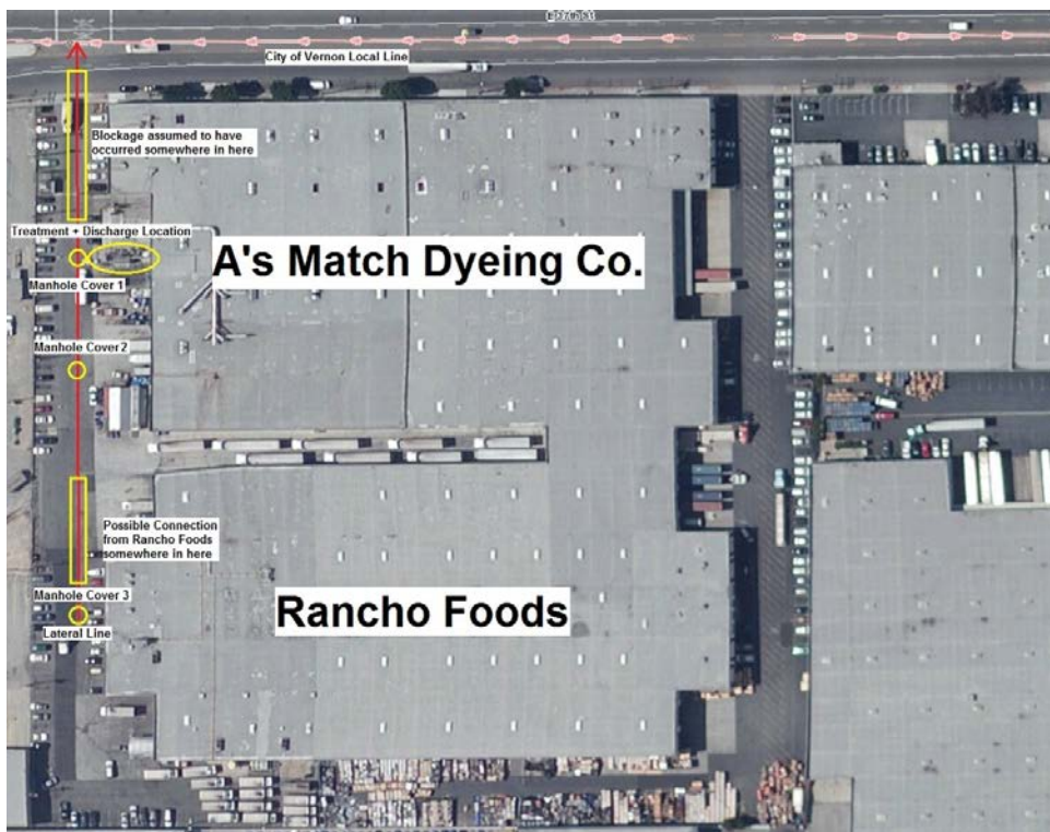
Figure 1: Area map showing the locations where Rancho Foods and A's Match Dyeing Company connect to the lateral sewer line.
