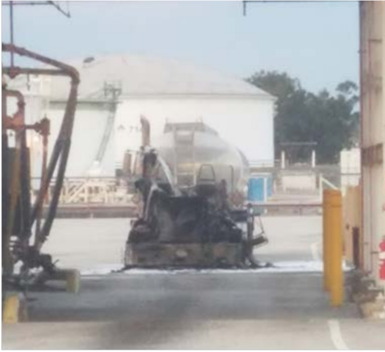
Figure 1: Burned truck cab at the Tesoro-East Hynes terminal truck loading facility.
