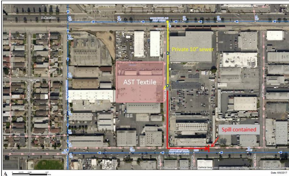
Figure 4: GIS diagram showing the location of the AST Textile Co., private sewer line (yellow line drawn in by Barnum), as well as the City (pink) and Districts' (blue) sewer lines in the area of the spill.
