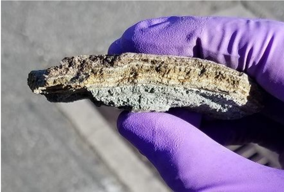
Figure 4: Profile view of one of the stones in Figure 3. Note the stratification that indicates long term scale build-up.
