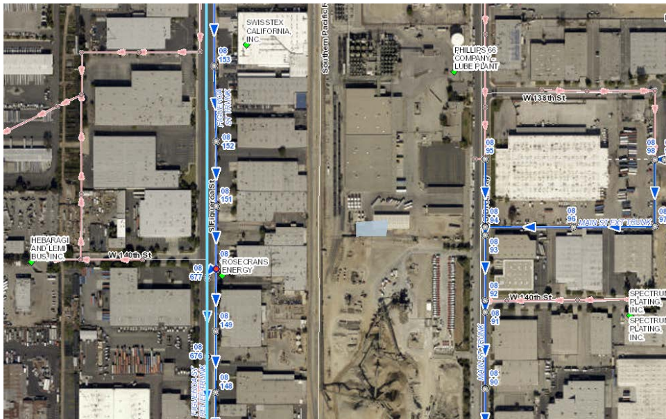
Figure 4: LACSD GIS screen grab showing the location of MH 08 0150 (red dot). Note the close proximity of the large Swisstex California textile dyeing facility and the Rosecrans Energy small oil lease.
