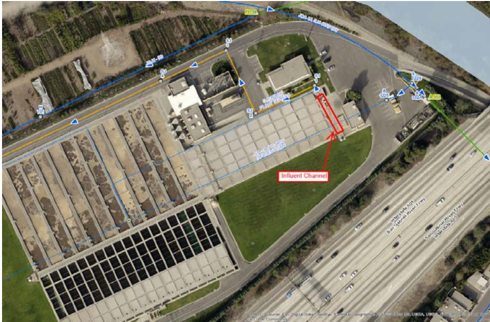
Figure 8: GIS view of the San Jose Creek West WRP showing the plant layout and the location of the influent channel where solids reportedly accumulate.
