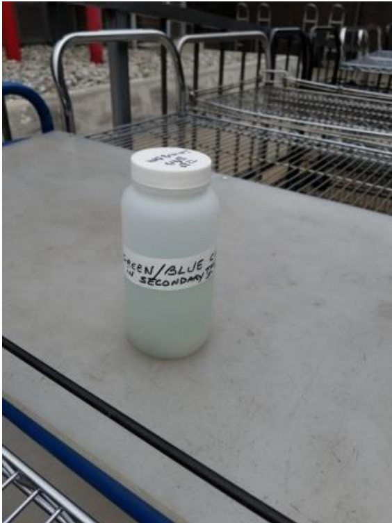
Figure 3: 5-9-18 WNWRP secondary tank grab sample. Note the blue green tint.
