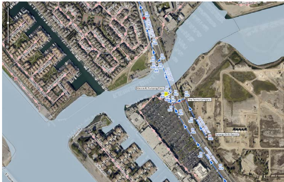
Figure 3: GIS map showing the area around the upstream of MH 03 0505, including the Marina #2 Pumping Plant and Section 4 of the Marina trunk sewer.
