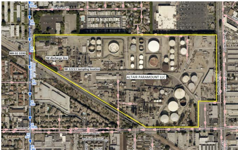
Figure 1: Annotated GIS diagram showing the relationship of the refinery, their industrial wastewater discharge line, and where it connects to the Districts' 15" Downey Ave Extension trunk sewer just north of Manhole (MH) 02 0390.
