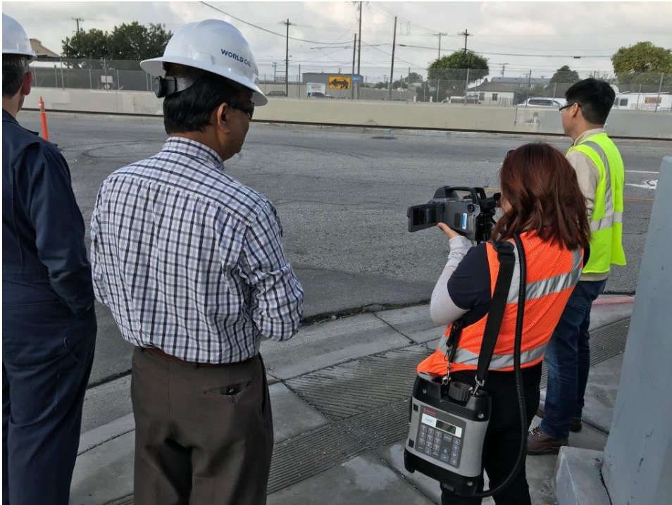
Figure 9: 3-24-18 SCAQMD Inspector Pham using a FLIR camera to detect the presence of headspaces gases emanating from MH 01 1463.
