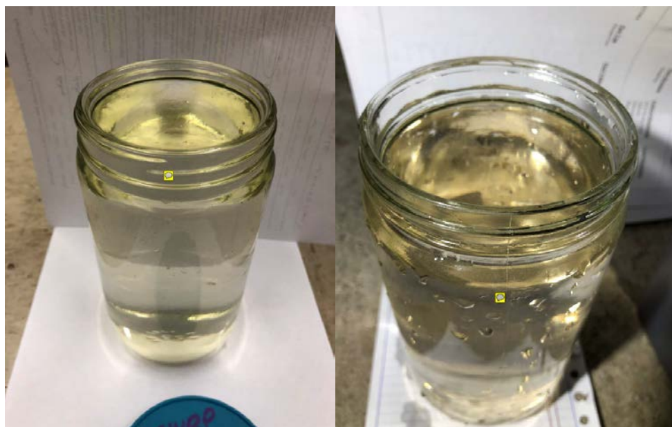
Figure 7: Side by side comparison of a grab sample of LCWRP final effluent on the left (taken at 00050 hours on 3-21-18 by Night team IW Inspector David Joh) and on the right a 50:1 diluted sample of the 1100-1200 hours 3-20-18 composite sample of effluent from Tri-Star Dyeing and Finishing.
