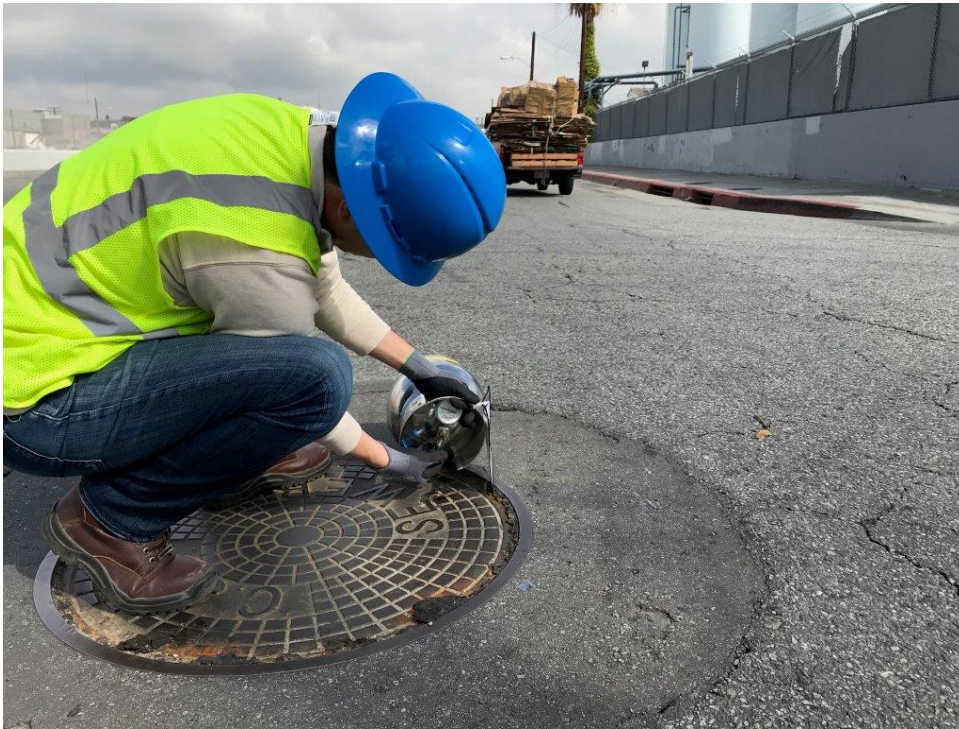
Figure 10: 3-24-18 SCAQMD Inspector using a stainless steel canister to collect a sample of the headspace gas emanating from MH 01 1463.
