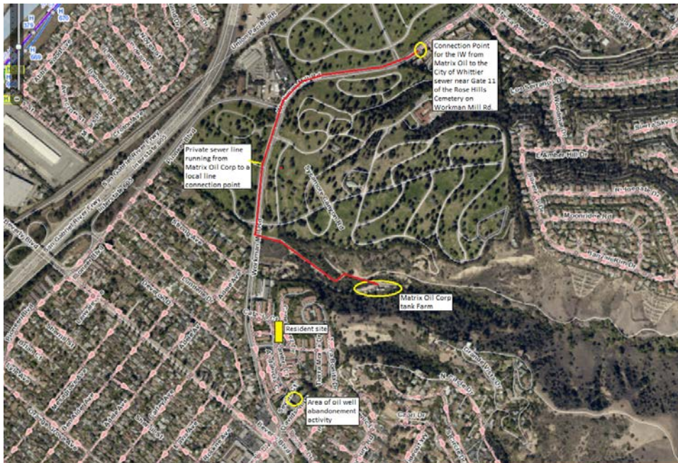
Figure 1: Annotated GIS diagram showing the location of the residence where the odor complaint and the locations of the oil abandonment project, Matrix Oil Corp., and sewer lines pertinent to the odor report.
